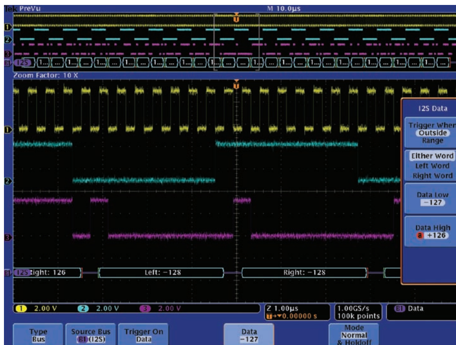
Figure 41. Triggering outside a range of values on an I 2 S bus.
