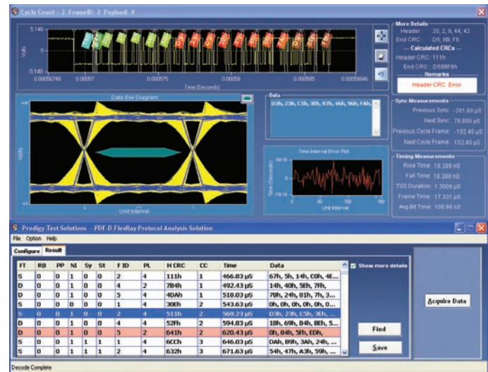
Figure 36. Eye Diagram analysis of a FlexRay signal.
