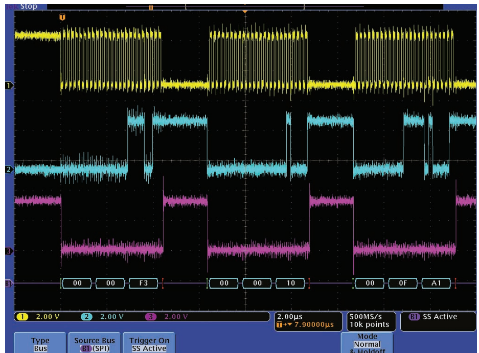
Figure 13. Correct synthesizer configuration messages.
