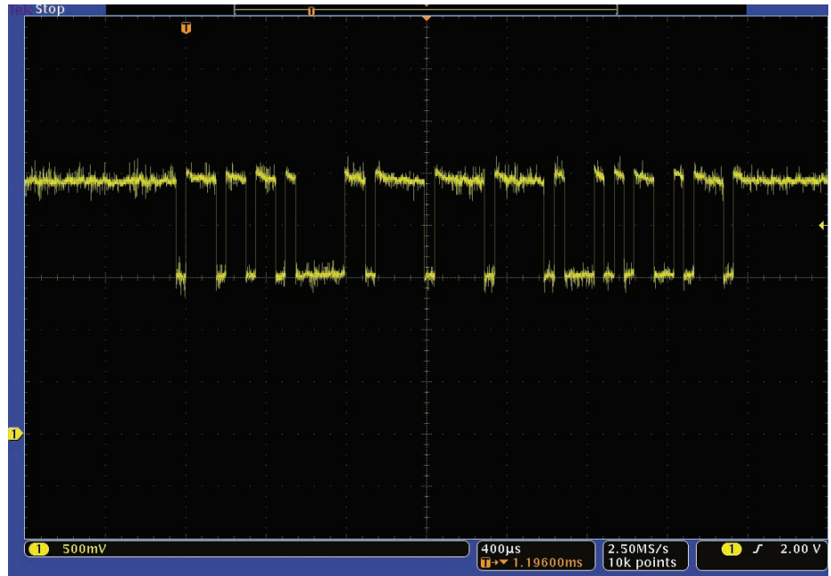
Figure 2. One message acquired from a CAN bus.
